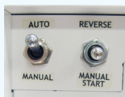
Can be operated by foot pedal or manual hand operation with a flip of a switch
