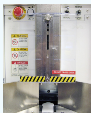
Protective Safety Cover, keeps your fingers safe and out of harm's way during use
